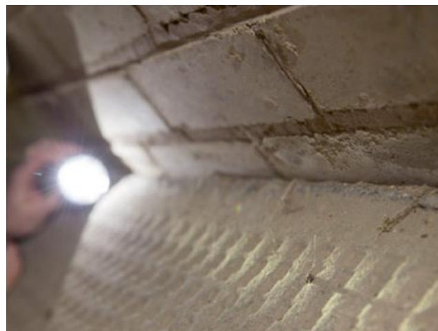
Figure A5.2 Diagram showing the effect of the low-angle torch in identifying dust particles
